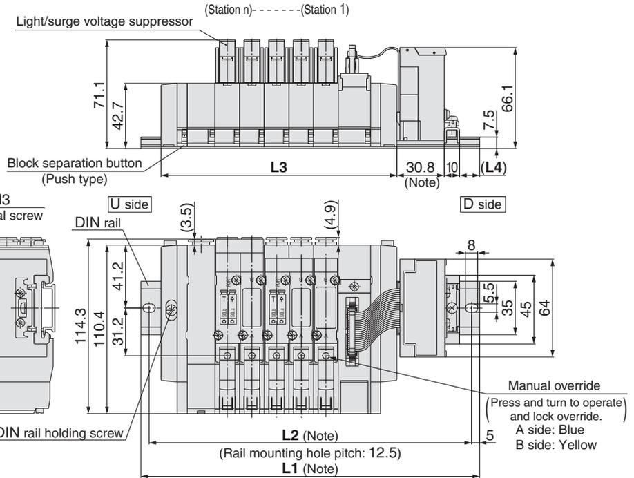
Note) The L1 to L4 dimensions of SS5Y5-45S1 □ D - Stations <sup>C4, N3</sup> D-C6, N7 are identical to those of SS5Y5-45S1 □ D - Stations <sup>C4, N3</sup> U-C6, N7.
