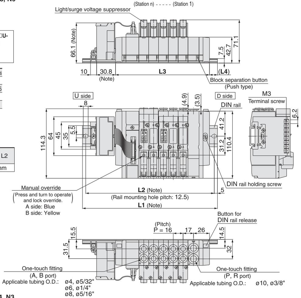
**SS5Y5-45S1□U- Stations B-<sup>C4, N3</sup><sub>C6, N7</sub>-Q (for SI unit types C, Q, R1, R2 and V)**
