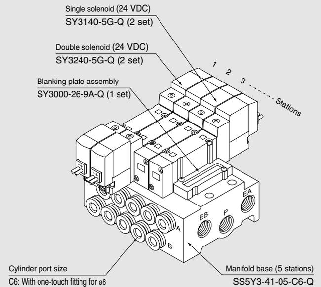
**SS5Y3-41-05-C6-Q 1 set (Type 41, 5 stations manifold base part no.)**
