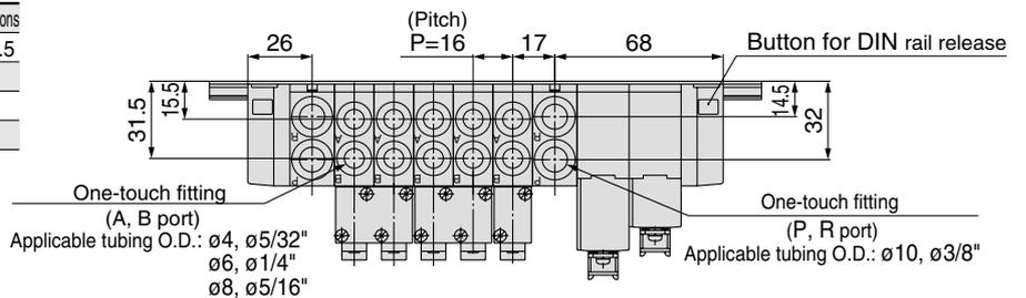
**SY5000: PC Wiring System Compatible (Flat ribbon cable/Plug-in)**
