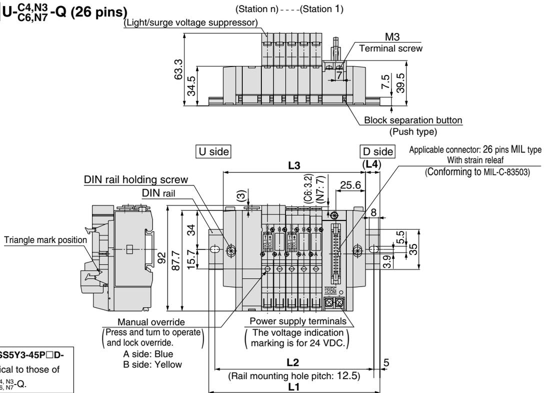
Note) The L1 to L4 dimensions of **SS5Y3-45P□D- Stations D-C4,N3-C6,N7-Q** are identical to those of **SS5Y3-45P□D- Stations U-C4,N3-C6,N7-Q**.
