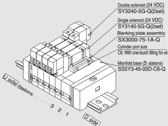
**SS5Y3-45-05D-C6-Q** 1 set (Type 45, 5 station manifold base part no.)
