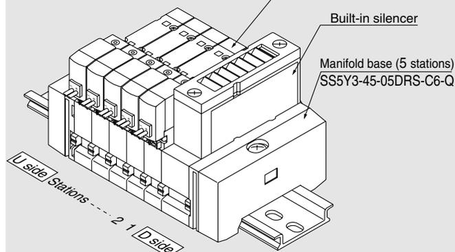
**SS5Y3-45-05DRS-C6-Q 1 set (External pilot specification with built-in silencer part no.)**
