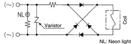
Note) Surge voltage suppressor of varistor has residual voltage corresponding to the protective element and rated voltage; therefore, protect the controller side from the surge voltage. The residual voltage of the diode is approximately 1 V.
