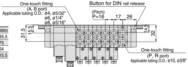
**SS5Y5-45T1U- Stations B-<sup>C4, N3</sup><sub>C6, N7</sub>-Q (18 pins)**
