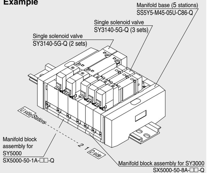
**SS5Y5-M45-05U-C86-Q 1 set (Type M45, manifold base part no.)**
