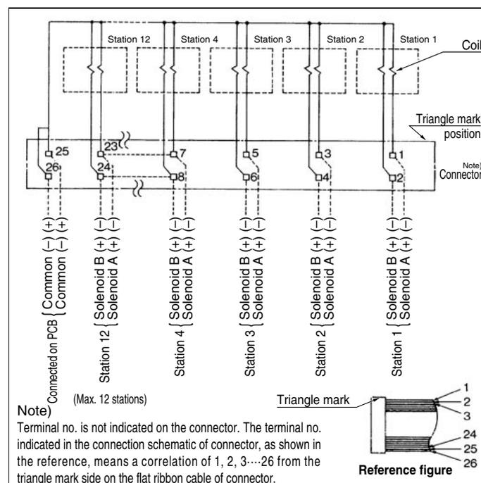
Note) Terminal no. is not indicated on the connector. The terminal no. indicated in the connection schematic of connector, as shown in the reference, means a correlation of 1, 2, 3...26 from the triangle mark side on the flat ribbon cable of connector.
