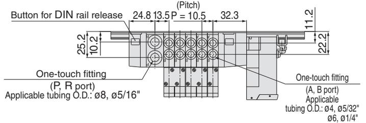
**SS5Y3-45S** □ - Stations **B**-<sup>C4, N3</sup>/<sub>C6, N7</sub> -**Q** (for SI unit types C, Q, R1, R2 and V)
