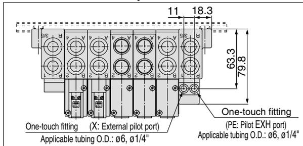
\* Air discharge port on the built-in silencer type and the external pilot's extracting position are in the D side.
