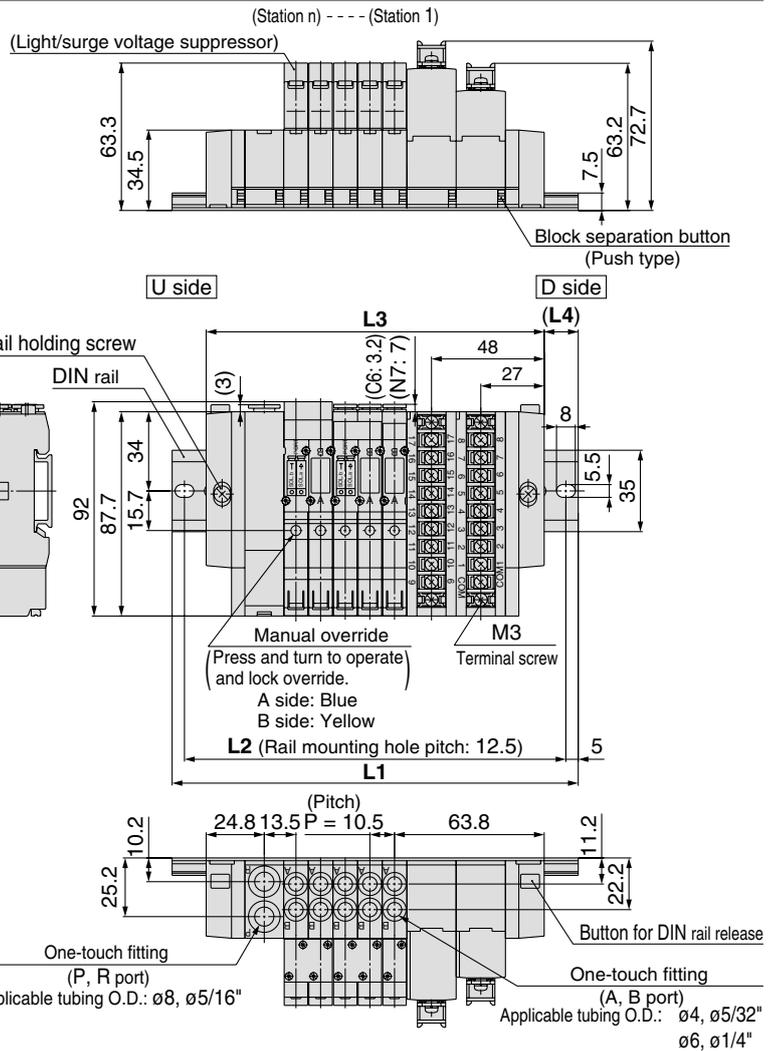
Note) The L1 to L4 dimensions of **SS5Y3-45T1D-Stations D-C<sub>6</sub><sup>4</sup>, N<sub>3</sub><sup>7</sup>-Q** are identical to those of **SS5Y3-45T1D-Stations U-C<sub>6</sub><sup>4</sup>, N<sub>3</sub><sup>7</sup>-Q**.
