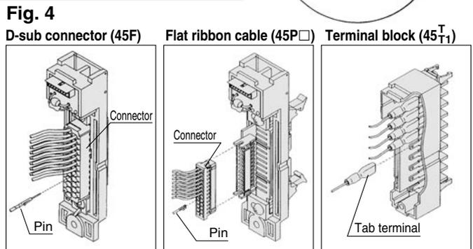
Note) After inserting pins, lightly pull lead wire to check that pins are locked.
