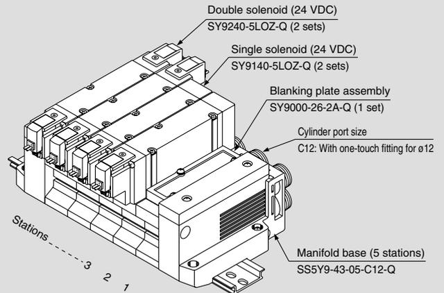
SS5Y9-43-05B-C12-Q 1 set (Type 43, 5 station manifold base part no.)
